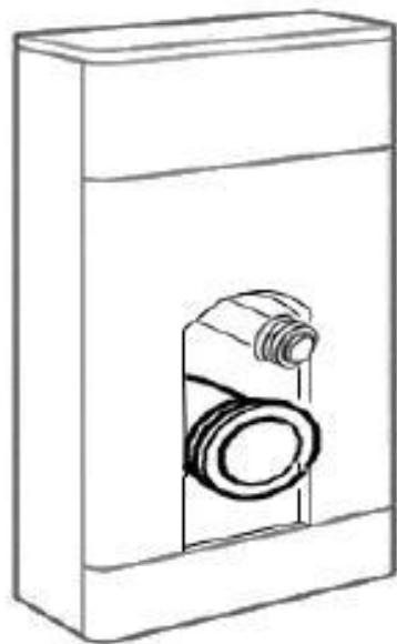
It is recommended to seal the cut edge and bottom edge of the unit, to protect against moisture ingress
